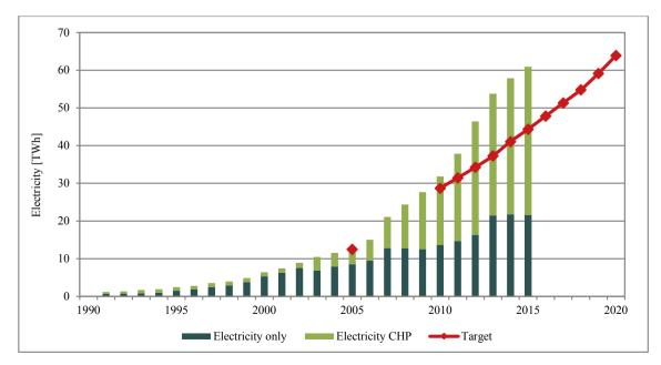
Fig. 9. Evolution of electricity production from biogas in the EU and targets [20,24,54].
