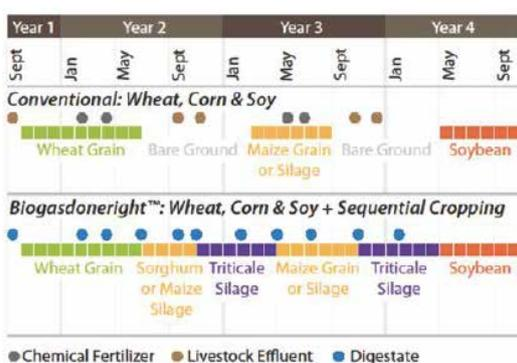
**Figure 3-3: Wheat-corn-soy 38-month cropping cycle showing Biogasdone-right® cropping systems with timing of mineral fertilizers, manure and digestate application (Valli et al., 2017; doi.org/10.1002/bbb.178)**
