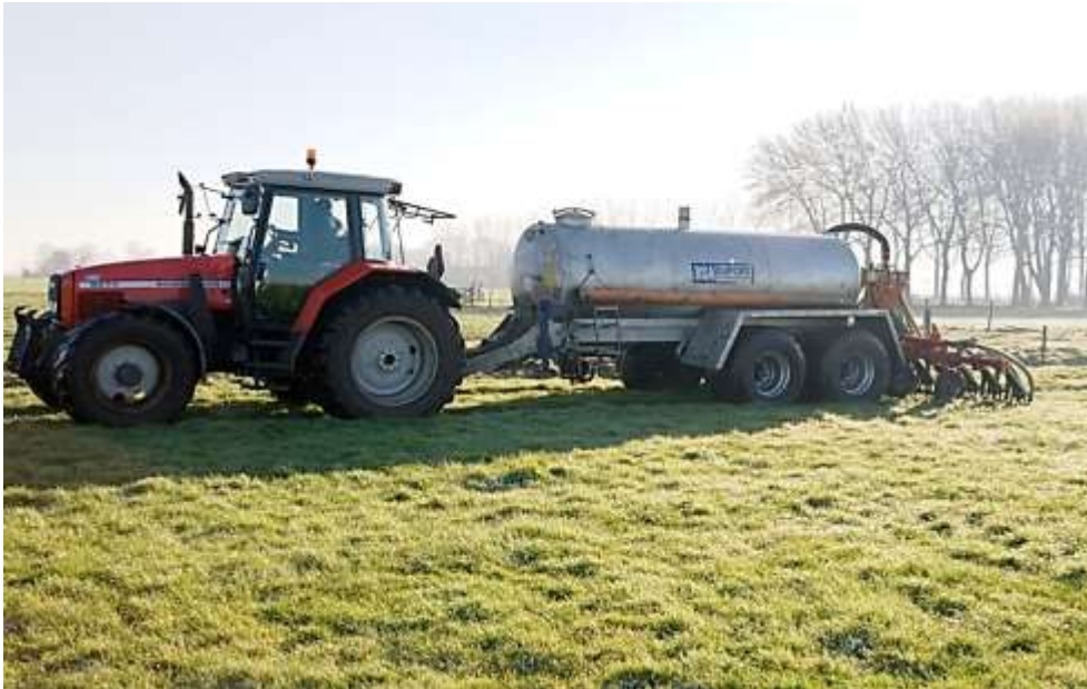
Figure 10 - Tanker fed sub-soil injection system.
