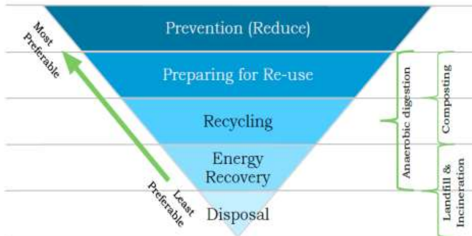
Figure 2 - The position of Anaerobic Digestion within the waste hierarchy (EU's Waste Framework Directive 2008/98/EC).
