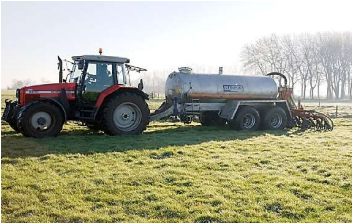
Figure 15 - Tanker fed sub-soil injection system.
