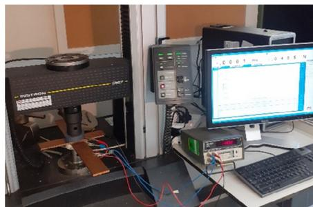
Fig. 2. Designed Set-up to measure EC of additives.
