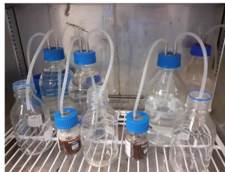
Fig. 1. Experimental setup of anaerobic digestion.
