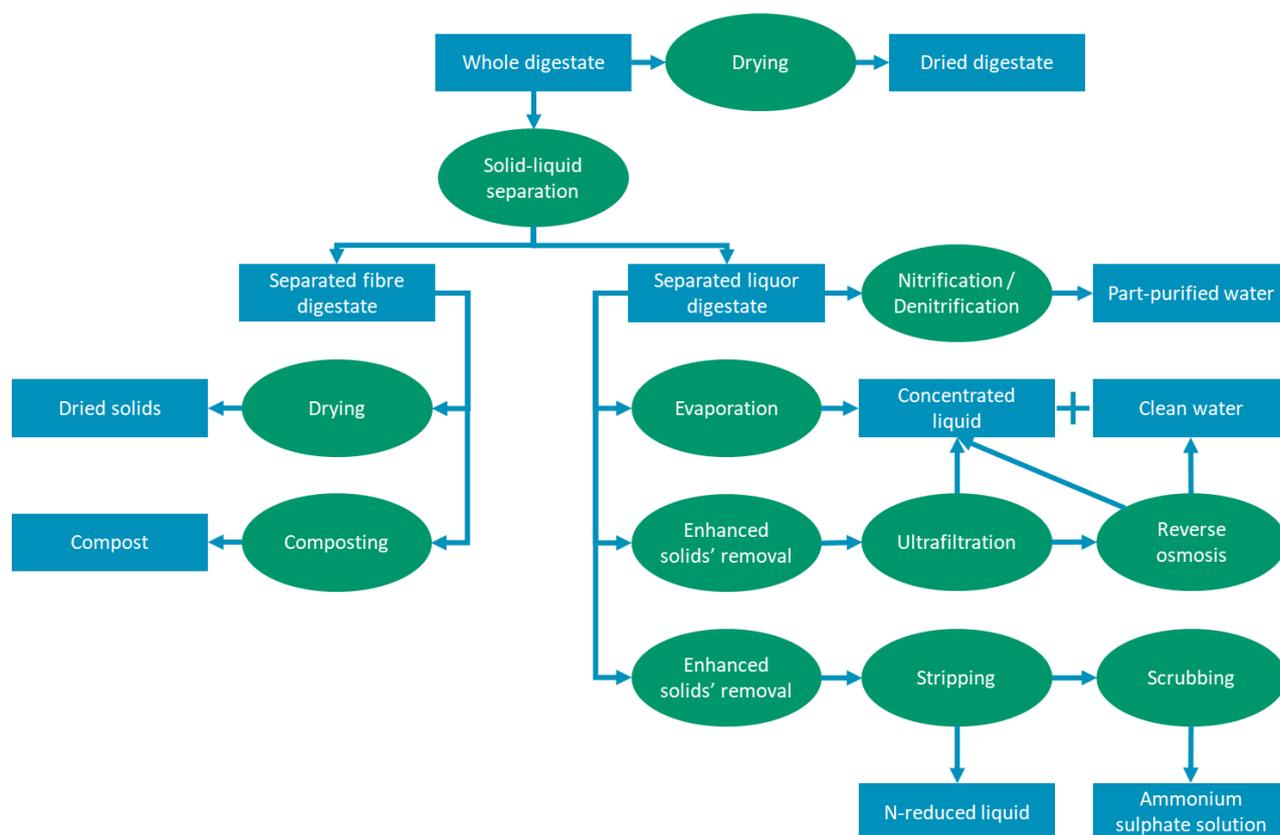
Figure 2 Overview of common digestate processing options. Adapted from Fuchs & Drosch (2013)
