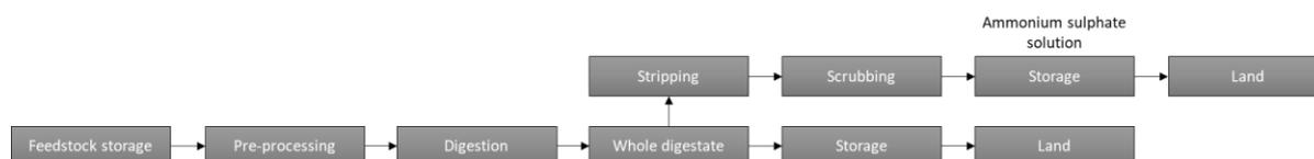
Figure 12 Process flow diagram for stripping of separated liquor
